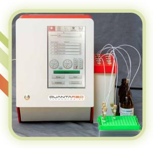
Some standard methods for urine analysis are using special reagents to transform the analytes to a detectable modification. Afterwards, a colorimetric measurement of the mixture is taking place. In contrast, the NUTRISHIELD Urine Analyser Prototype is planning on not using any chemical reactions and therefore not needing any reagents. This facilitates a user friendly and safe operation. Apart from this advantage, the goal of the protoype is measuring two health indicators at once.
